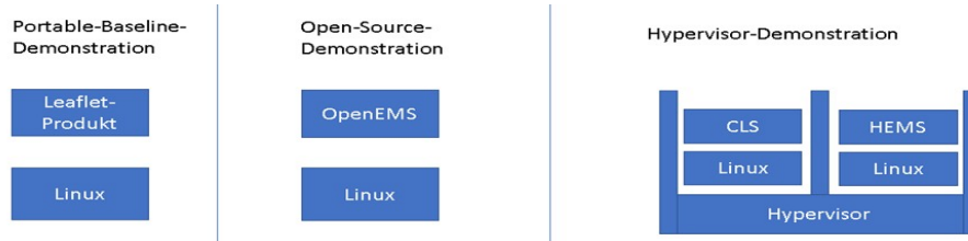
Figure 24: Software stack for the three sub-demonstrators
